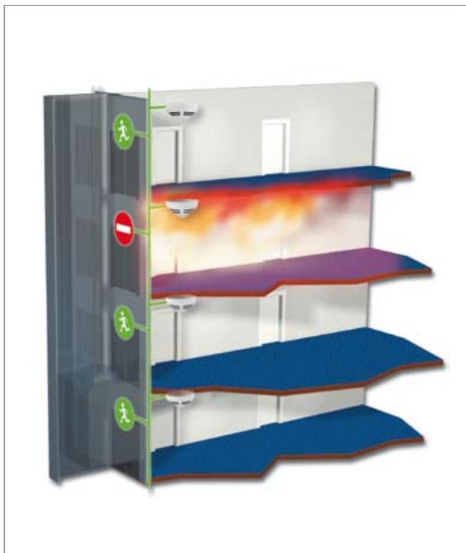
Above: Swift closure of automatically controlled fire protection doors prevents the further spreading of smoke as well as the spread of fire.
